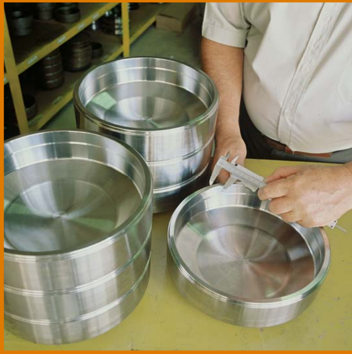
Micron Mill incorporates a fixed 8000 g “ring and spigot” bowl
