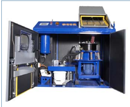
Micron Mill incorporates a fixed 8000 g “ring and spigot” bowl
